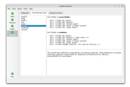
The workflow icons (left hand side) include a step for "Topology". Within this step, you would review the topology findings (automatic recognition) for the following:
