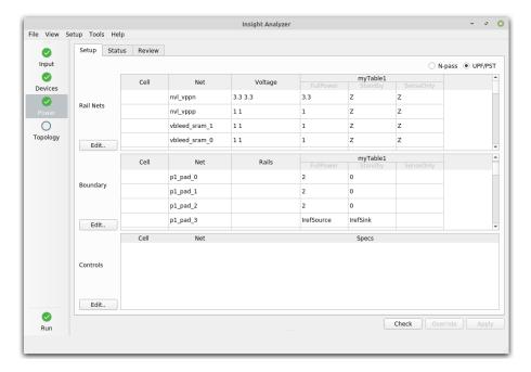
A notable application of this states association is in the Analog Floats checking. In all prior Insight Analyzer versions, floats would be detected in a kind of wildcard fashion, where it was not possible to lock down specific input combinations that were known to be prevented externally. Now, in v5, you define the valid external state combinations, such as an I-ref-source that will be provided as long as analog power is valid.
